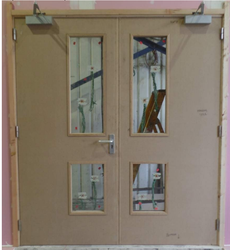
Exposed face – pre test
